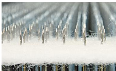
1 pav. Adatinio veltinio gamyba („Horizon-Felt Industrial Group“, 2022)
