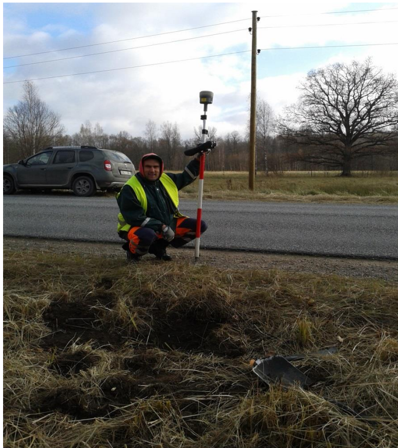
Figure 1. GPS mobile receiver Trimble R10 GNSS (from the personal archive)
